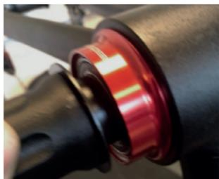
b. Align and press into bearing
