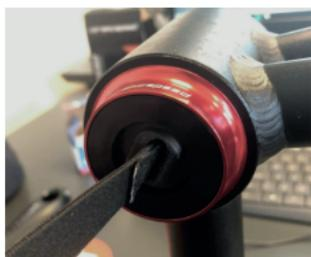
b. Engage the chip inside the dust cover
