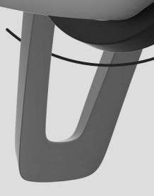
PLACE THE FROG ON YOUR HANDLEBAR, SEATPOST OR ANY TUBULAR STRUCTURE ON YOUR BIKE, STRETCH THE STRAPS AROUND THE TUBE AND LATCH ON TO THE HOOK
