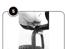
Installing the **Spider Rack Cradle** to the top or side of your Spider Front Rack is easy. Simply unscrew the 4 screws within the cradle with 5mm allen key, locate the male and female part of the cradle on the **spider front rack** tube and screw **cradle** back together.
