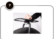
Installing the **Spider** Pannier Receiver is easy. The Spider Pannier Receiver mounts to the top of the **spider front rack**. Simply unscrew the 4 screws within the pannier receiver with a 5mm allen key, locate the male and female part of the pannier receiver on the **spider front rack**.
