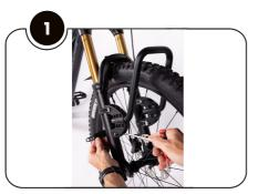
Position the **straps** on your front forks and connect the hole in the strap with the lug in the **feet**. Note the 2 holes in the straps. Choose the hole that best suits the thickness of your front forks. Once the **feet** are roughly in place, start tightening the **straps** using the allen key in the 4 bolts as shown in the next step.
