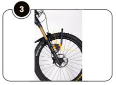
Depending on the size of your front forks/Bike, you can loosen the bolts shown above and slide the **spider front rack** into the attachment foot to suit preferred location, and then tighten the bolts again.
