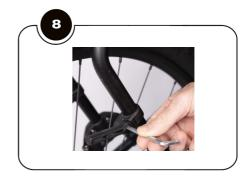
To install the lower pannier catch **anti-sway ingers**, loosen the **anti-sway finger** bolt so you con pull the clamp of the antisway finger apart enough to slide onto the **spider front rack**.
